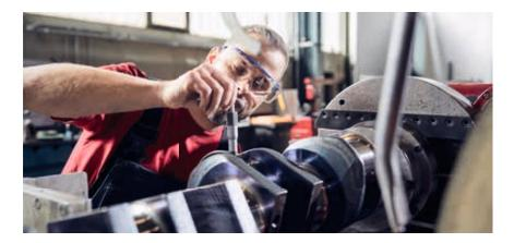
Depending on the manufacturer's specifications, a general overhaul may also involve the reuse of engine components. Our workshop technicians dismantle the engine, clean all components, examine them for damage, and measure them for wear according to the manufacturer's specifications. If the parts are undamaged, still within the manufacturer's tolerances, and therefore suitable for overhauling, we shall consult with you on the extent of the work in detail.
